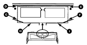
3. Verify exhaust adaptor (with damper) is squared up in house duct and lines up with holes in mounting plate.
